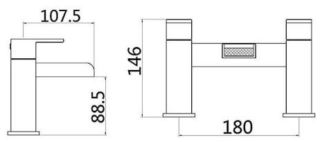
All Dimensions are in millimetres. The information contained on this page was correct at date of issue. Fitting dimensions are provided as a guide only. Some variation may occur due to manufacturing tolerances. We pursue a policy of continuing improvement in design and performance of our products and so reserve the right to change specifications without prior notice.
